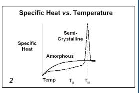
They have a broad softening temperature ( $T_g$ , glass transition temperature) range (Figure 2) that allows the material to soften gradually, melt and flow without prematurely solidifying. These polymers generally are very efficient with regard to their ability to transmit ultrasonic vibrations, and can be welded under a wide range of force/amplitude combinations.
